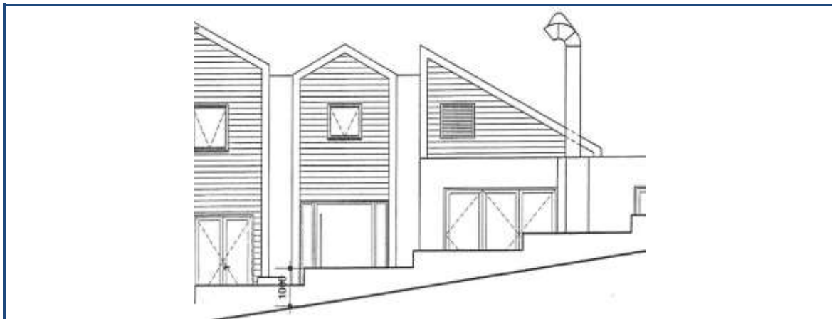
Separating mono-pitched roof with flat roof elements
